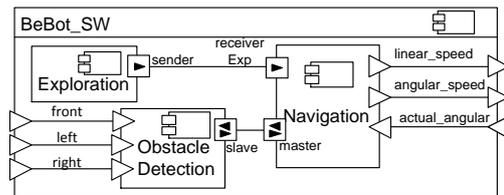
Figure 3: Component Type of the BeBot Software
