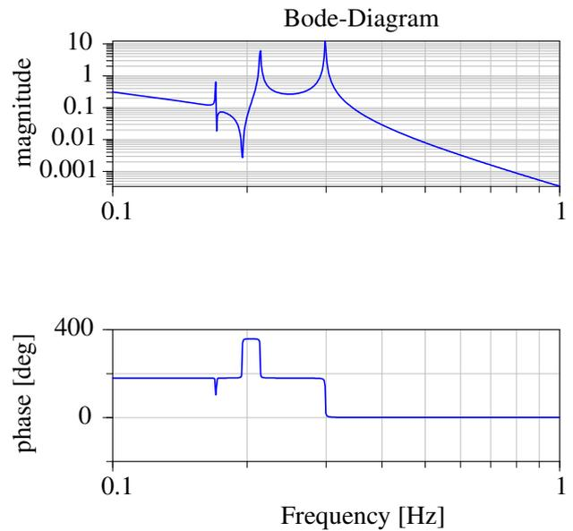
Figure 12: Bode-Diagram of the epicyclic gear from Figure 8 with reduced stiffness of one of the gear contacts.
