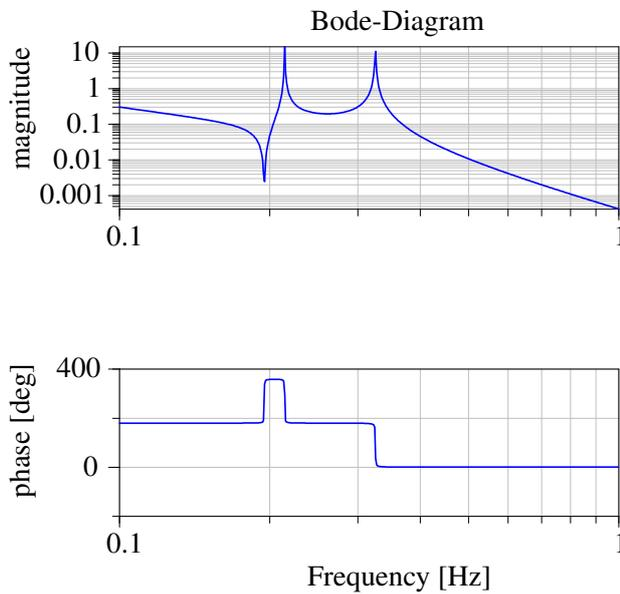
Figure 11: Bode-Diagram of the epicyclic gear from Figure 8
