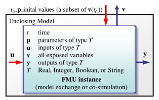
Figure 2: Data flow between the environment and the FMU Blue/red arrows: Information provided by/to the FMU.
