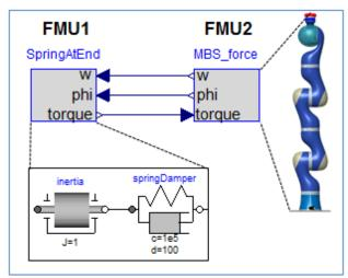
In multi-body system terminology, this is called a "force element". Typically, FMU 1 would be a complicated device, e.g., a controlled electrical motor with a gearbox, but the essential part is the force element at the interface. The inputs to FMU 1 are the angle phi and the angular velocity w of the end point of the spring/damper system. The output would be the torque generated by the spring/damper. It is calculated with the simple equation
