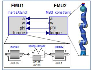
Since FMU 1 is connected to a joint of FMU 2, the coupling leads to a constraint equation that states that the angle of the revolute joint of FMU 2 is identical to the angle of inertia2 in FMU 1. It is well-known that such a model cannot be transformed by purely algebraic transformations into a state space
