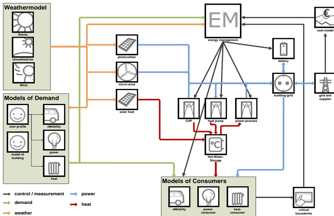
This paper describes the approaches and philosophy of the library by using a CHP powered building with stationary battery. One of the shown examples is the search for an optimal solution between stationary battery cost and renewable coverage of the vehicle mileage in a typical commuter driving cycle.
