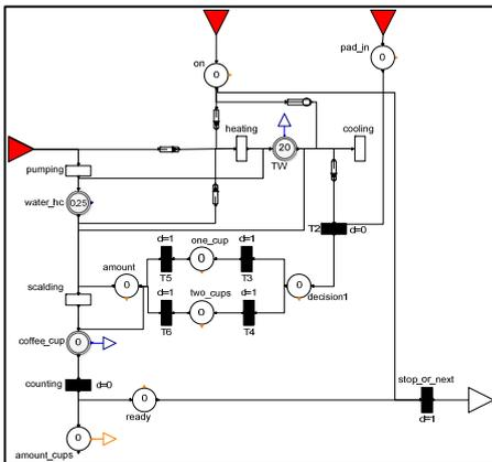
The first example demonstrates the representation of functional principles by a model of a Senseo coffee machine and the second one is a model of a printing production process. The third example presents the applicability of modeling business processes. All models are provided as application cases in the library. Additionally, the application of the PNlib for modeling biological processes has been already shown, for example, in [2].
