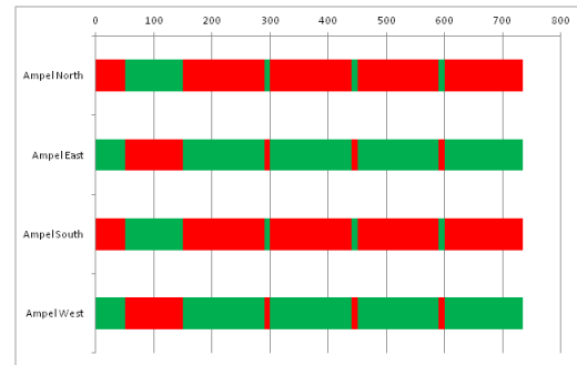
Figure 13: The signal time plan the alternative control algorithm given by (14) in Modelica.
