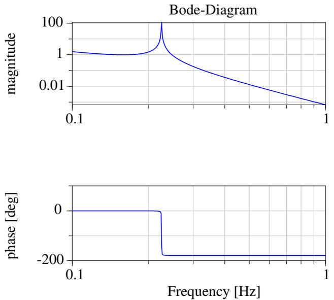
Figure 10: Bode-Diagram of the spur gear from Figure 6
