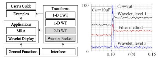
The results showed significant advantages of the wavelet method over filtering. As shown in the figure, the wavelet method obtained a much stronger pulse and a more significant magnitude change related to a fast drop of 20% capacitance.
